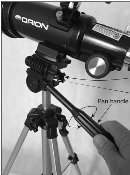
**Figure 12.** Use the pan handle to smoothly move the telescope horizontally and vertically.
